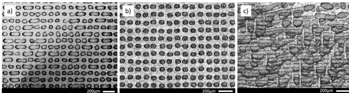
Fig. 10. Single splats of INK<sub>SiO<sub>2</sub>CMC</sub>: (a) without heating of the substrate, (b) with the substrate temperature of 50 °C, (c) after 3 passes of printing with the substrate temperature of 50 °C.
