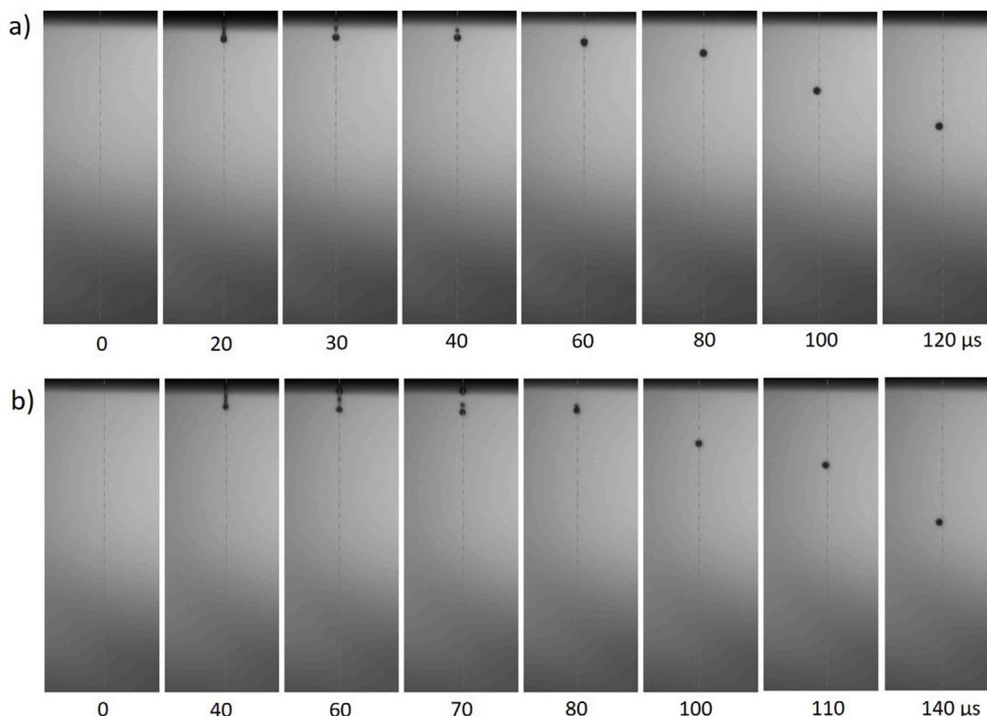
Fig. 6. Drop generation process with optimal parameters registered frame by frame for: (a) INK<sub>SiO<sub>x</sub>CMC</sub>; (b) INK<sub>SiO<sub>x</sub>PEDOT</sub>. The dotted line indicates the nozzle central axis.
