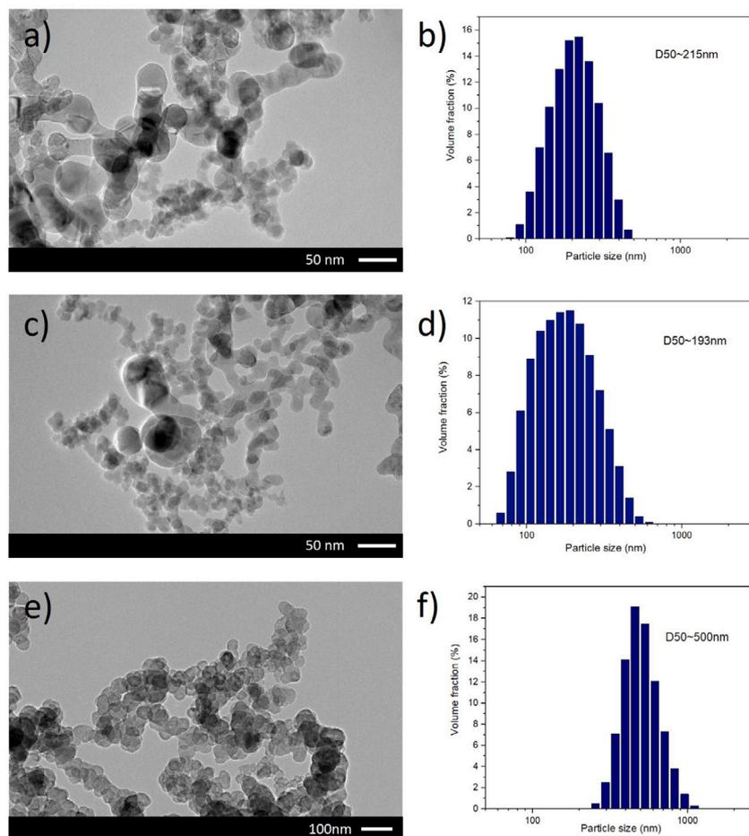
Fig. 1. Morphological characterization and particle size distributions of powders: (a), (c), (e) TEM images of Si, Si $\Omega$ C, and CB powders, respectively; (b), (d), (e) Particle size distribution obtained with DLS technique of Si, Si $\Omega$ C, and CB powders, respectively.
