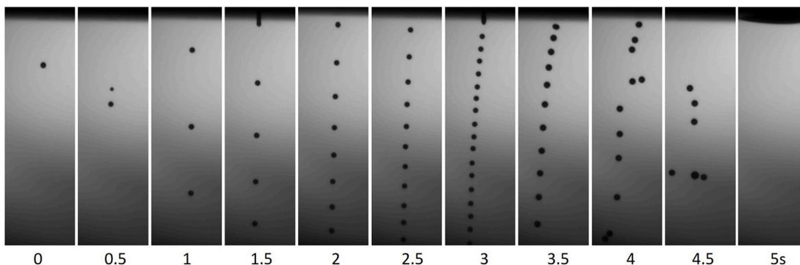
Fig. 7. Ejection process of INK\_SiO<sub>2</sub>\_CMC when increasing jetting frequency from 100 Hz to 1000 Hz.
