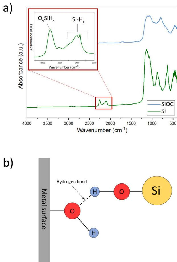
Fig. 9. (a) FTIR spectra of Si and SiO<sub>x</sub> powders, (b) Schematic representation of hydrogen bond between Si particle and metal surface possibly causing the ejection issue.
