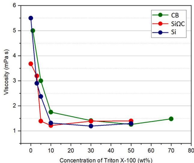
**Fig. 3.** Determining the optimal dispersing agent concentration: viscosity as a function of Triton X-100 concentration for Si, Si $\Omega$ C, and CB powders (1.5 wt% of powder in DI-water), measured with the rheometer Fluidicam.
