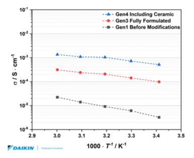
and discharging processes. Going through several generations, we were able to obtain materials with best-inclass values for their ionic conductivity. Unusual values for fluoropolymers were obtained by tailoring the salt-to-plasticizer-to-matrix ratio and in particular through ceramic additives, which enable a substantial increase in conductivity even when used in small fractions.
