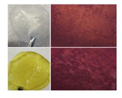
The aim of the plasticization is to decrease the temperature of the high conductivity range of the hybrid polymer electrolyte used in all-solid-state lithium-ion batteries. This would allow much higher currents (higher power) to be available for electric vehicles powered by the batteries.
