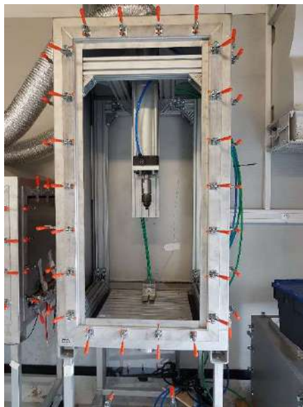
Figure 7: Safety machine for nail penetration tests
