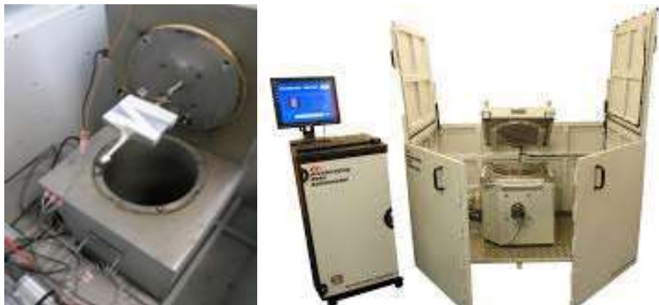
Figure 8: Photographs of the calorimeters used at CEA to perform thermal runaway tests
